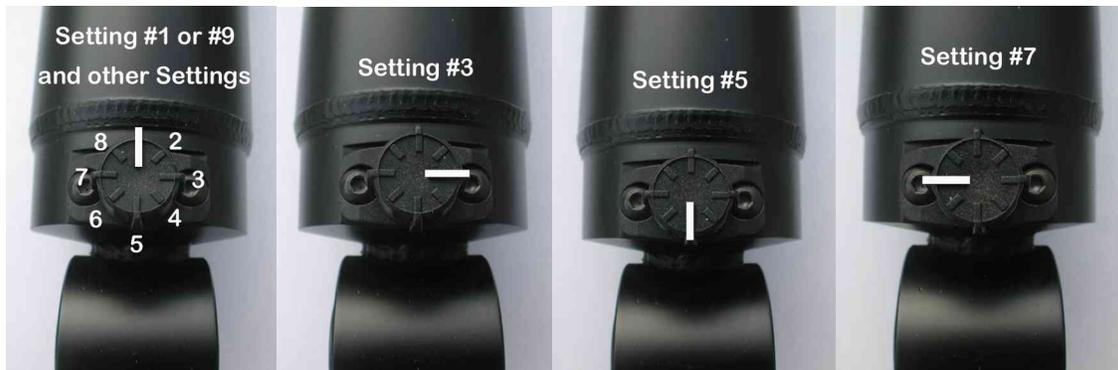
GT shocks for the H1 have 9 possible damping settings, starting with the lowest setting, which is #1, not “0” as many have assumed.
